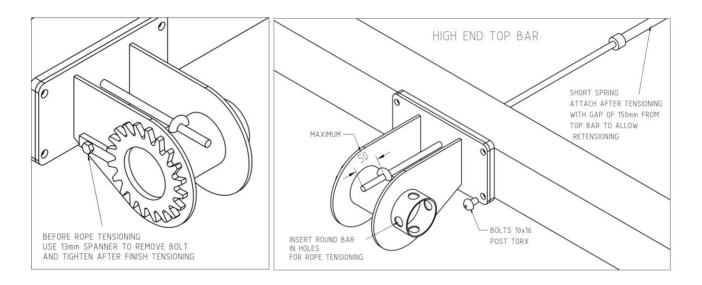
It is important to not over tension the cable and or tension when not required. The playground standard allows a minimum clearance from seat bottom to finished soft fall level of 400mm and a maximum of 1900mm.
